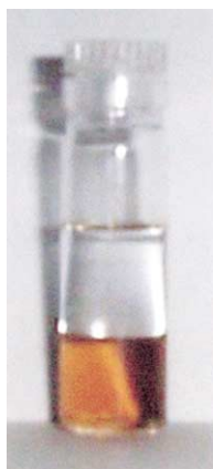
Figure 1. Retention of catalyst in fluorous phase (orange) after hydroformylation below the colourless organic phase (toluene/aldehyde).
